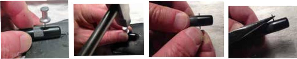
Remove the securing pin by hand; gently tap with a hammer; the final removal involves pressing out and using pliers
