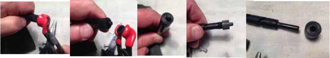
With the pin removed carefully ease off the blind cap exposing the mid section with seal housing- pull out the spiral shaft; you are now ready to start restoring! ;
