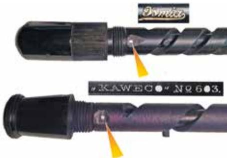
Once the seal is exposed the procedure for restoring, any safety pen is exactly the same as the Montblanc. However the design differences of turning knobs, connecting rods and spirals can create uncertainty unless you know what is inside.
